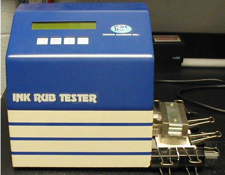
Figure 4: Modified Ink Rub apparatus used for the cloth abrasion test
